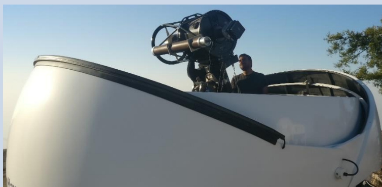
Figure 1: The complete telescope assembly of 43cm telescope, kept inside 12ft Astro-Heaven dome.
