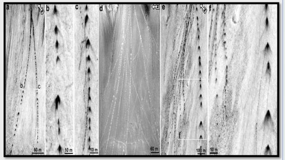
**Figure**: Formation of boulder track with ejecta. a-c, Boulder fall ejecta with a diverse spread of ejecta along the track. d, multiple boulder tracks with light toned ejecta. e, the ejecta spread along the track varies. f, spacing between the bounces and ejecta spatial spread varies and small sub-tracks from some boulder bounces. All images have an applied stretch to best highlight the BFE.
